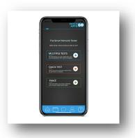
Patch App & Go T1 is the one man Data Continuity Tester and Cable Tracer, powered by any mobile device running on android or IOS.
