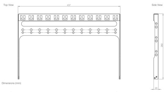
Zettonics TEN<sup>21</sup> blank, for blanking off any unused slots in Zettonics TEN<sup>21</sup> 1U and 2U Chassis.
